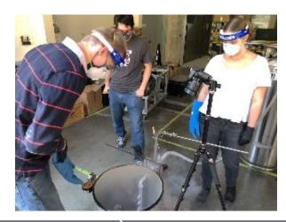
Preliminary Tests: Proved our system was viable for further testing.. Liquid Cryogen Sprayer: Average of 97.0% removal by mass with ideal parameters
